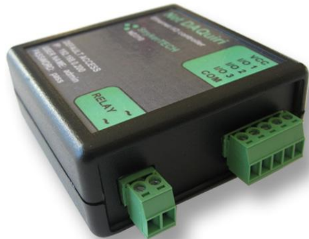
Figure 2 - Back side view, terminal blocks.
